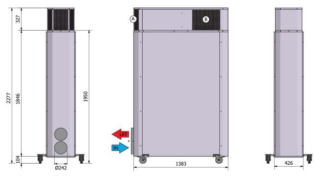
A = Recirculation air supply B = Air discharge \* The unit can also be supplied with the connections on the right side.
