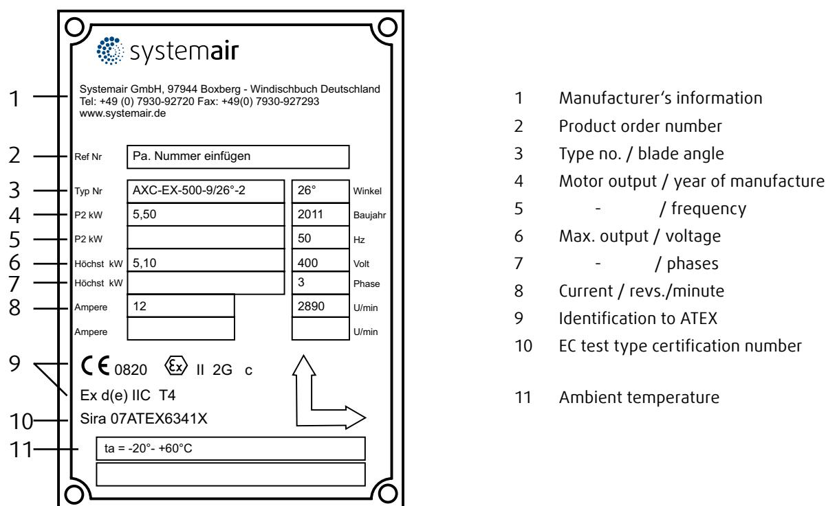
Fig. 4: Name plate of the AXCBF-EX / AXC-EX series
