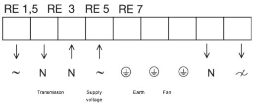
Transmisson:between ~ and N is always 230V when the transformer handle is in pos. 1-5
