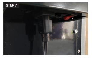
Connect the C13 power cable to its receptacle, then connect the power cord to a power outlet.
