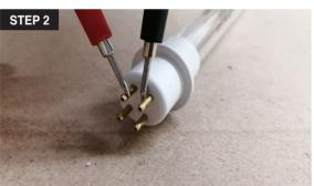
2. Placing the probe of the ohmmeter to one of the four pins on the end of the lamp, touch the other probe of the ohmmeter to each of the other pins until you find the matching pin.
