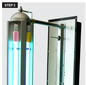
5. Adjust the UV lamp assembly so it will be positioned in the middle of the duct. The arms that support the lamp assembly have an adjustable clutch which allows the lamp and extrusion to be set at a distance from 10" to 15" from the backplate
