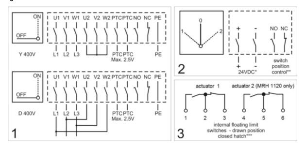
Diagram 1 (connection of electric motor in the fan's service switch)
