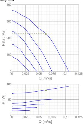
Name: KVK 125 INS. CIRC. DUCT FAN | Item no.: 2430 | Version: 50 Hz
