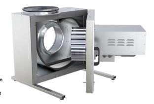
The KBT fans have a swing-out door for easy inspection and service. The fan is isolated from the casing via connectors and anti-vibration dampers are incorporated into the base frame.
