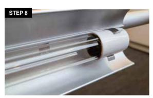
8. Rremove the UV Lamp from its packaging. Then, while wearing the included cotton gloves, carefully "clip" the UV lamp using the metal spring clips into the parabolic reflector.
