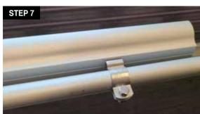
Slide the two parabolic reflector clamps over the support rod to position them. Insert the bolts and nuts and tighten everything with a socket wrench.
