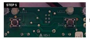
5. Then press on the reset button for resetting lamp timer to zero.
