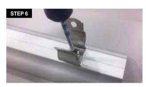
Attach the clamps to the back of the aluminum reflector using Phillips screws and blocking washers. The parabolic reflector holes are predrilled and pre-threaded.
