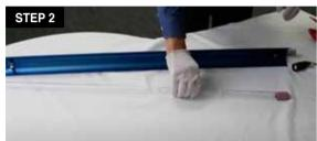
2. Release the old lamp from the reflector brackets and remove it.
