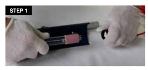
1. Disconnect all power before performing any maintenance or service. With the power off, remove the lamp from the reflector and unplug it.
