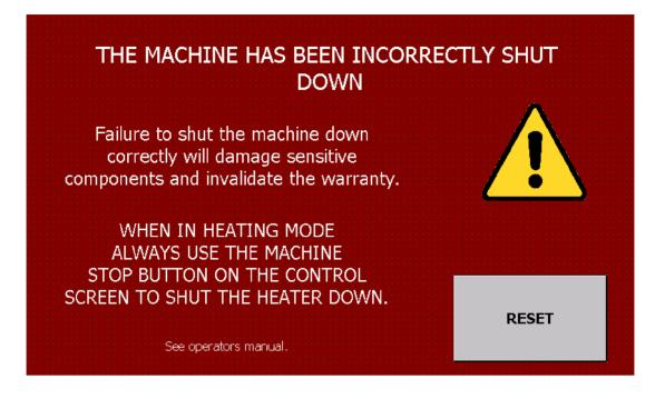
The incorrect shut-down fault has activated. This indicates that the last time the machine was used the correct shut-down process was not followed.
