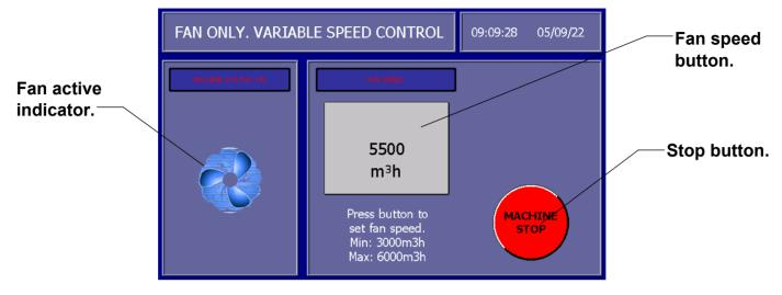
To change the fan speed press the Fan speed button. A key pad will appear.
