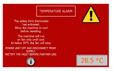
The safety limit thermostat has activated. This indicates excessive temperatures within the heater.
