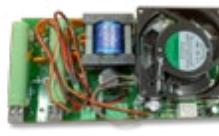
The HT Board is equipped with voltage control. An anomaly alarm is triggered below a certain threshold. This alarm is visible on the LED display.
