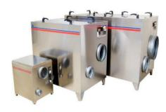
**DehuTech™ 400** desiccant dehumidifier is delivered as a complete unit with fans, filter, rotor and controls. The dehumidifier is ready for site installation and connection to standard-size ducting and electrical mains (1 x 230V 50Hz).
