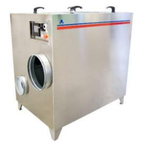
**DehuTech™ 3500** desiccant dehumidifier is delivered as a complete unit with fans, filter, rotor and controls. The dehumidifier is ready for site installation and connection to standard-size ducting and electrical mains (3 x 400V 50Hz).
