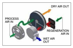
is drawn into the dehumidifier, where is passes over a wheel impregnated with Silica Gel. As the air passes over this wheel, any moisture present in the air, is absorbed into the Silica Gel wheel before leaving the dehumidifier as warm dry air.
