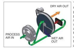
The Silica Gel wheel is continually, slowly rotating, typically at three revolutions per hour. As the wheel rotates a small portion passes through the regeneration segment. During this phase a second air stream (Regeneration Air) is heated to a high temperature before passing over the wheel. Any moisture present in the wheel is released into this air stream, this hot wet air is then exhausted outside the area being dried.
