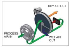
The Silica Gel wheel is continually, slowly rotating, typically at three revolutions per hour. As the wheel rotates a small portion passes through the regeneration segment. During this phase a second air stream (Regeneration Air) is heated to a high temperature before passing over the wheel. Any moisture present in the wheel is released into this air stream, this hot wet air is then exhausted outside the area being dried.
