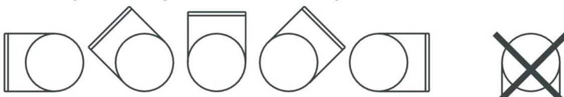
4. The access opening to a room must be equipped with a fixed mesh or an intake air device which makes it impossible to touch the heating elements.
