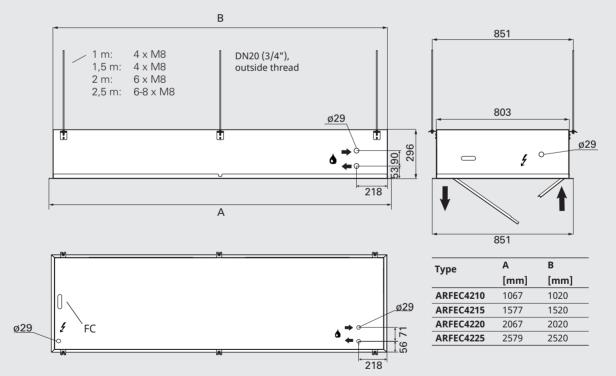
Minimum distance from outlet to floor for electrically heated units is 1800 mm.
