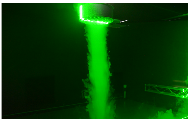
Fig. 1: Air flow visualisation (left: vertical discharge pattern; right: horizontal discharge pattern)
