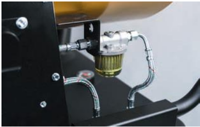
Fuel preheater is inside, fuel filter is outside
