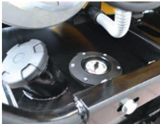
A leakless fuel tank closure and a big fuel level indicator.
