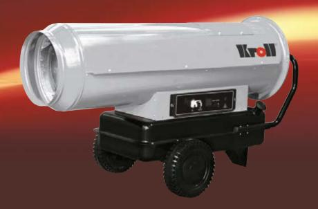
Oil heaters without flue gas pipe. They are suitable for outdoor use or in well-ventilated rooms and have a degree of efficiency of 100 %. Fuel supply from the integrated tank via an integrated compressor with the models "GK". With the models "GP" via an integrated high-pressure pump.
