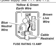
connected, that the cable outer insulation extends beyond the cable restraint and that the restraint is tight.
