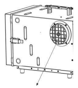
NOTE: When using a long tube or covering the outlet, the warning light (filter light) can be lit.
