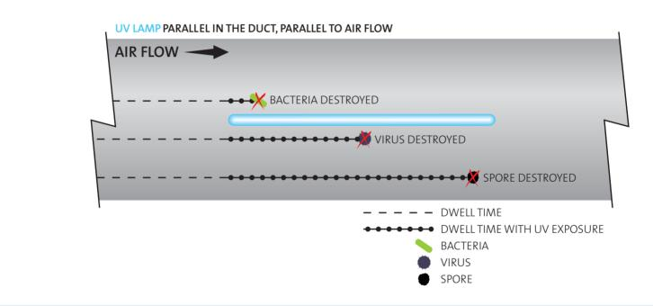
Sanuvox proprietary Mercury Vapour Ultraviolet Lamps produce two UV wavelengths. UVC (Germicidal 254nm) and UVV (Oxidizing 187nm) pure fused quartz glass that are combined into one single UV Lamp emitter.
