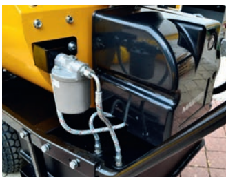
The heater gets the fuel from the tank below but can also be connected to an external tank
