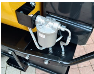
Fuel filter is outside. Fuel pre-heater is inside, within the combustion head
