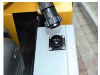
The motor is connected to the electronic panel with a snap-on connector, allowing an easy maintenance
