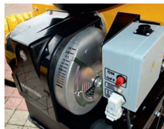
Control panel including: On/off switch with light messenger, reset button, socket for remote thermostat: Analog or digital
