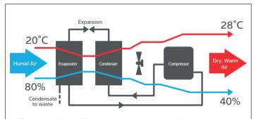
The process of dehumidification involves moisture-laden air being drawn into a dehumidifier where the air passes across a refrigerated coil. The air is rapidly cooled below its dew point, condensing the water vapour and recovering its latent heat energy for re-use. The cooled air is then passed across the condenser where it is reheated and returned to the served area at the required lower relative humidity.
