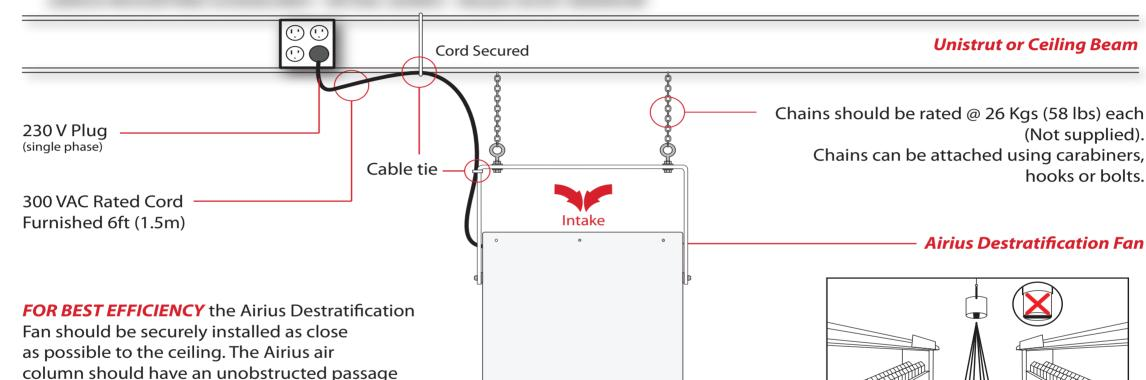
Unit should be positioned with exhaust nozzle parallel to aisle.
